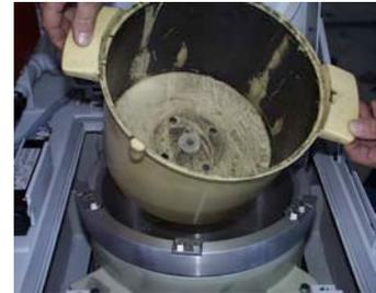
The high-speed aluminium rotor guarantees filtration quality. The heavy duty plastic sludge basket facilitates simple operation.
